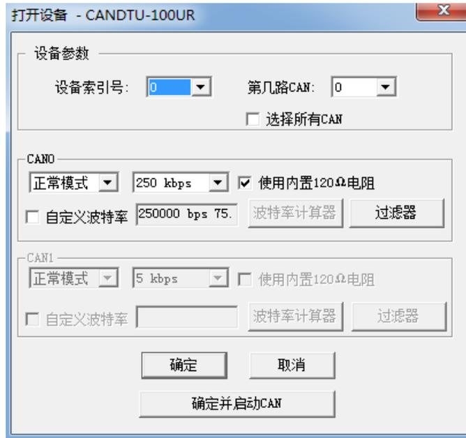
Figure 5.6 Setting CAN parameters
